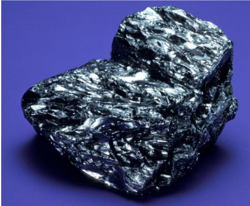
Figure 7. This is an example of foliated graphite from Saint Lawrence County, New York. Image is from Smithsonian National Museum of Natural History Department of Mineral Sciences Collections.
