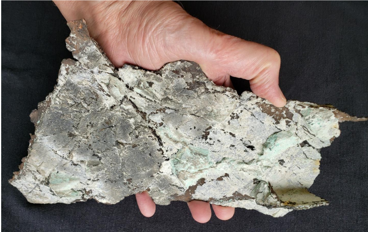
Figure 4. This flat plate of native copper is formed by the leaching of copper-bearing sulfides, where the dissolved copper moves downward and redeposits as native copper at the water table. The flat aspect develops because the copper is precipitating along fractures within the rock. Note the “fin” of copper in lower right, indicating a perpendicular fracture also hosting part of the copper. Specimen is from the Chino Mine, Grant County, New Mexico.
