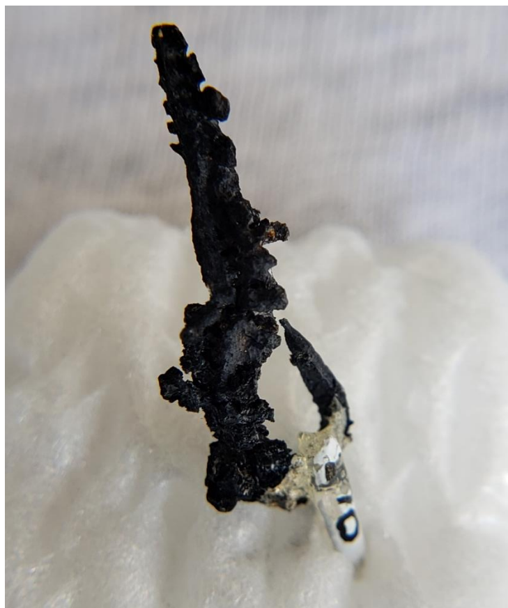
Figure 2. This is an example of the tarnish coating that develops on native silver when exposed to the Earth's atmosphere. This tarnishing is the reason true silverware had to be polished frequently. The jagged surfaces shown along the edges of this specimen are called hackly fracture. From Mexico, this specimen is 0.8 inches long.
