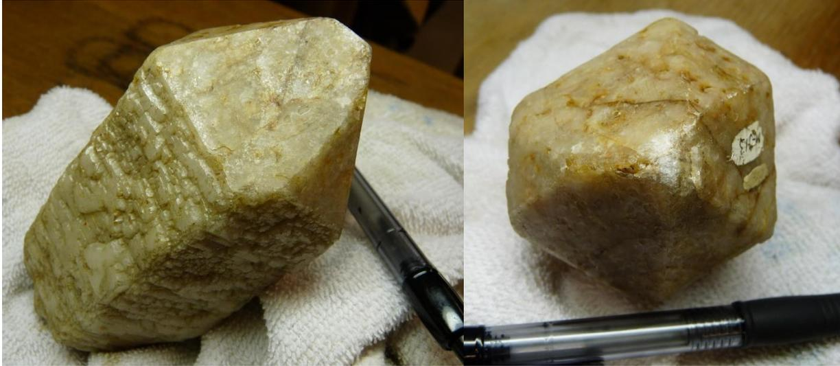
Figure 3. This is an excellent example of a hexagonal quartz crystal showing the characteristic six-sided form when viewed along the long axis. Note that not all crystal faces have to be the same width in order to create the hexagonal shape.
