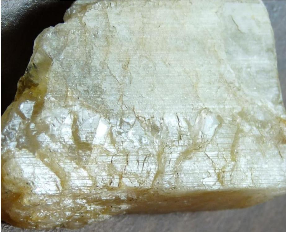
Figure 2. This is a crystal of plagioclase with well-developed *striations* on the lower half of the specimen. These are observed as very fine dark lines as light is reflected off this cleavage surface. Length of crystal is 1.6 inches.
