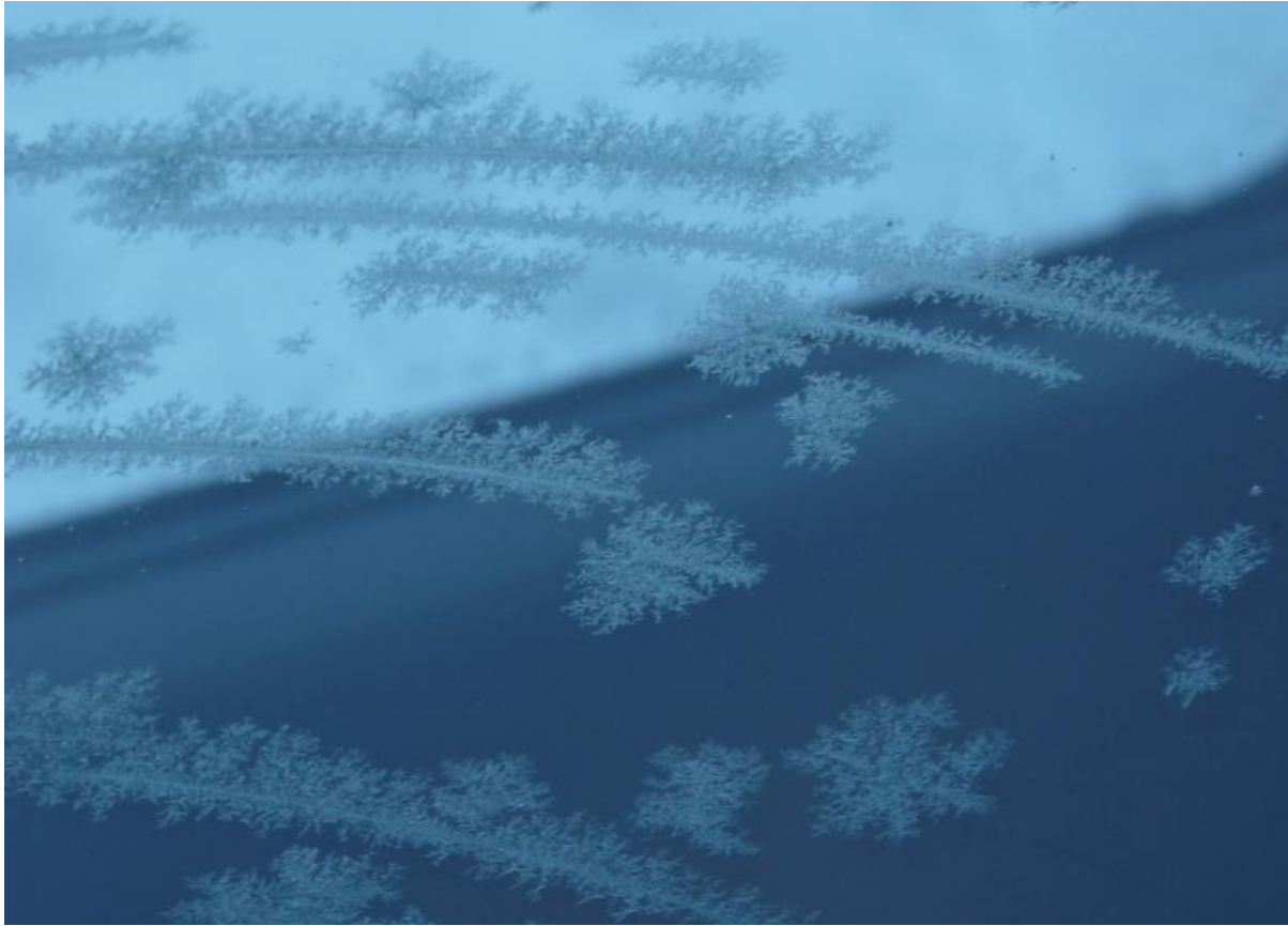
Figure 2B. A close-up view of the windshield in Figure 2A showing how ice prefers growing outward from the initial sites of nucleation along the streaks, rather than starting new nucleation sites scattered randomly all over the glass surface. This pattern of mineral growth is referred to as a dendritic habit.
