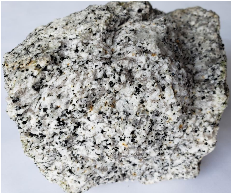
Figure 2. This is a typical specimen of granite. Visible mineral includes feldspar (white), quartz (gray), and biotite (black). The small patches of yellow to brown stain represent biotite flakes that are beginning to break down due to weathering, resulting in iron oxide staining. Width of this specimen is about 4 inches. Rock is from Boise County, Idaho.
