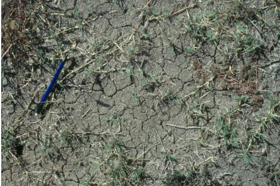
Figure 5. The abundance of polygonal cracking in the surface of this soil indicates the presence of significant smectite clays. This swell-and-shrink property often results in cracking of concrete slabs and roadways. Note mechanical pencil for scale.
