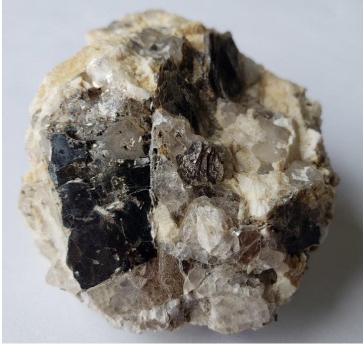
Figure 1. Biotite flakes (black) in a piece of granite create a strong color contrast with the other minerals present, which include quartz (gray) and feldspar (white). Width of specimen is 2.2 inches. Rock is from Boise County, Idaho.
