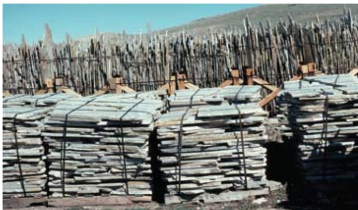
Large, flat plates of quartzite up to 3 m in diameter and approximately 1.5 cm thick ready for shipment; plates are stacked vertically to minimize breaking. This quartzite has a global market for veneer building stone. Middle Mountain, south-central Idaho.
