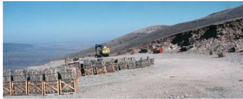
Looking north at typical Quarry on the west side of Middle Mountain. Note that the pallets have plates of quartzite stacked both vertically and horizontally. The large plates must be packed vertically to avoid damage during shipping.
