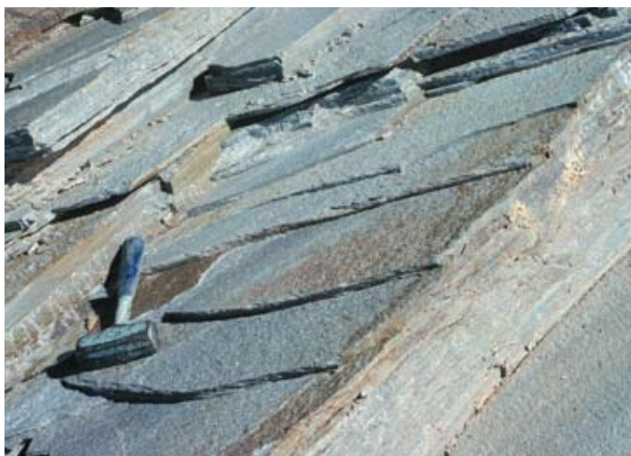
Quarry where quartzite is easily split along spaced cleavage. Note the large muscovite mica grains exposed on the well-defined cleavage surfaces. The cleavage is consistently spaced at 1 to 2 cm throughout the exposure. The cleavage is exceptionally well developed where parallel to bedding. Middle Mountain, south-central Idaho.
