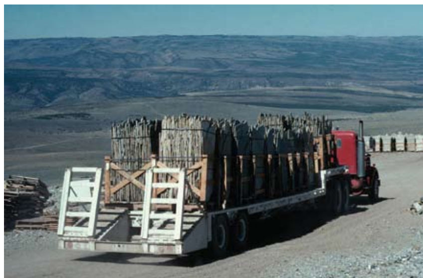
Truck hauling pallets of platy quartzite building stone from the quarry. Plates up to 8 feet in diameter can be transported if they are stacked vertically.
